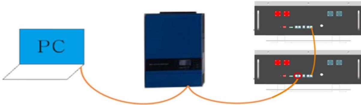
Note: When the single unit is used, the inverter communicates with the battery as the host;
